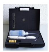
The **ZESTRON® Resin Test** visually and temporarily identifies the local distribution of resin-based residues on electronic assemblies via a color reaction. Critical resin residues, which cause poor adhesion of conformal coatings and delamination effects can be localized during the production and removed by a cleaning step. Thus the critical resin amount of <40  $\mu$ g/cm² (258.06  $\mu$ g/sq in) according to J-STD 001 can be met.
