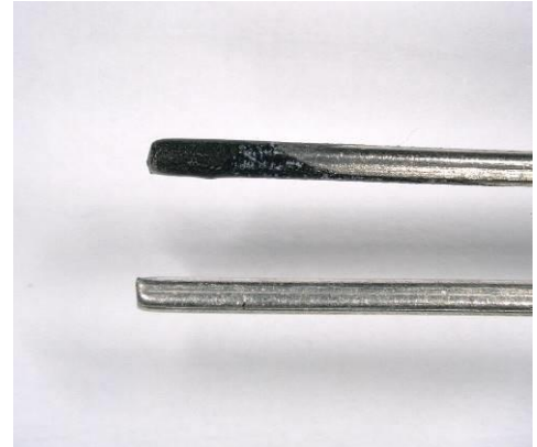
Above: Reaction with test (good solderability) Below: No reaction with test (bad solderability)
