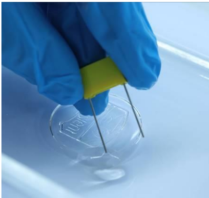
Immersing a THT connector in the test fluid
