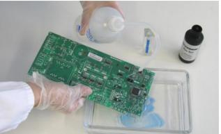
Rinse thoroughly with distilled or DI-water. It is recommended to conduct the test over a laboratory bench or sink.
