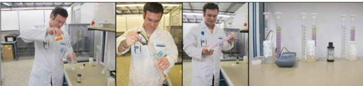
Figure 3 – Example of measuring with the Bath Analyzer 20 at Rohde & Schwarz: 1. Pouring cleaning bath sample into cylinder, 2. Adding test fluid, 3. Shaking the cylinder, 4. Brief wait, followed by determination of concentration level according to phase separation
